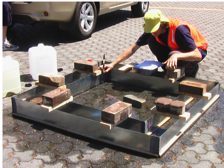
Figure 4. Double Ring Infiltrometer (all dimensions in mm).
