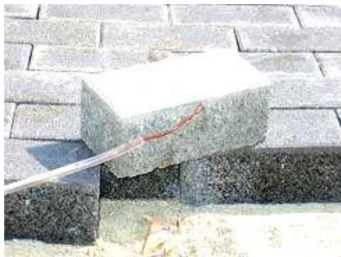
Figure 1. IL block specimen installed with Type-T thermocouple.
