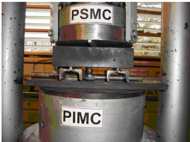
Figure 6. Flexural test of mortar samples according to the proposed IRAM 11656 Standard.
