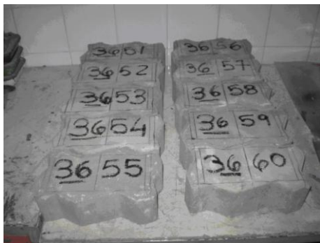
Figure 1. Pavers with the inscribed rectangle marked for bending test.
