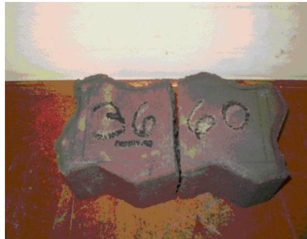
Figure 10. Rupture of a Uni-Stone paver under flexion.
