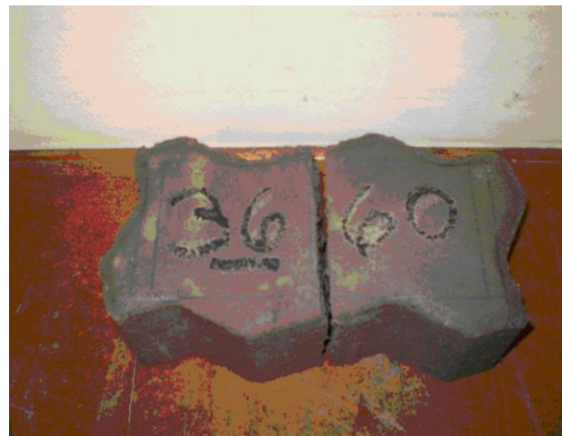
Figure 10. Rupture of a Uni-Stone paver under flexion.
