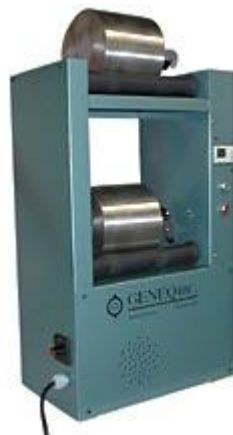
Figure 1. The Micro-Deval test apparatus (Source: Geneq, Inc.).
