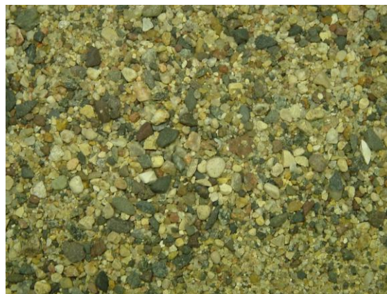
Figure 3. Example of sand from the ICPI bedding sand test program with a total combined % of sub-angular and sub-rounded particles equal to 65% according to ASTM D 2488 [ICPI, 2004].
