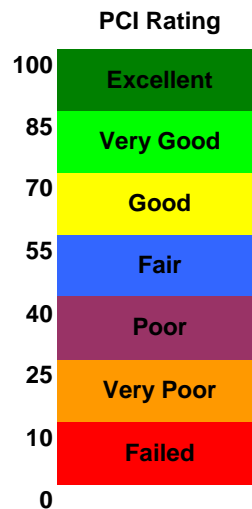
Figure 3. Level of Service Based on Pavement Condition Index.
